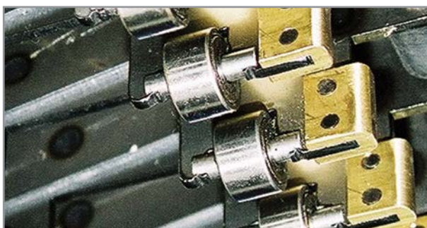
Supporting rollers with lateral brass guides
