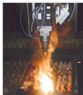
Material load test - laser beam path and burning behaviour
