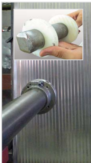
Impact test on covers under DIN EN 12417
