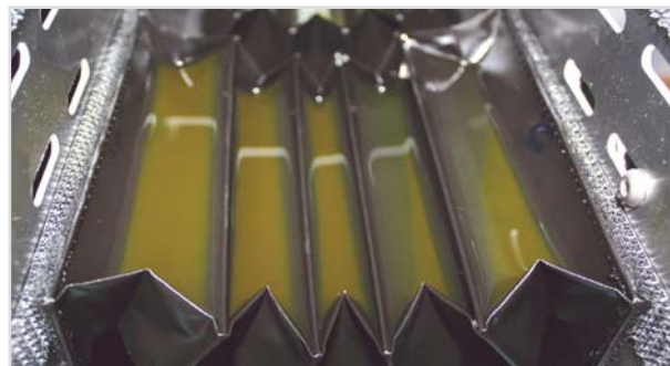
Static material load test - tightness test
